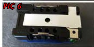
In **PIC 6**, the gasket leaves the bottom outlet's ground tab exposed. This will result in an un-grounded top outlet, and a grounded bottom outlet.
