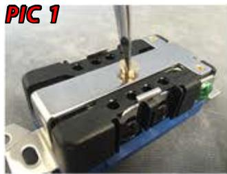
**Step 1.** Remove the center screw from the back of the outlet.
