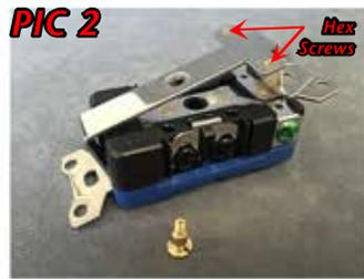
**Step 2.** Pry the mounting bracket off of the outlet.
